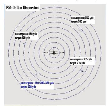
Note that the further away the target bullseye is, the larger the hit area, despite the target being in convergence distance each time.
