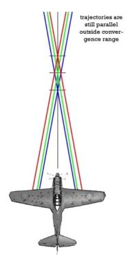
When staggering the convergence, you have two options. You can do it as in the picture to the right and have the inside guns set furthest out. This will give you an additional point of converging bullet streams (of one wing only) at a relatively close range. I have found this setting to be useful in MG armed planes, when I know I'll be fighting close range and take some of my shots up close, inside convergence range.
