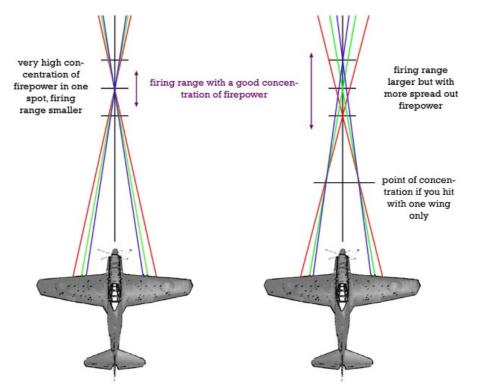
You can also stagger your convergences. Keep the distances close though - as in 250 on the outer pair (red), 275 on the middle pair (green) and 300 on the inner pair (blue). Staggering has the advantage of a larger firing range, but the concentration of bullets overall is not as good.
