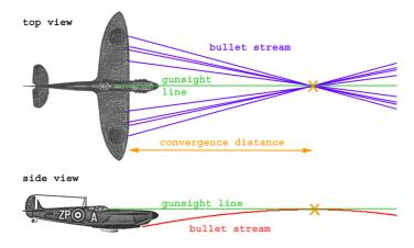
rounds meet (converge) in the orange X, a point at *convergence distance* on the gunsight line. The pilot can now use his pipper to aim. Also note that the rounds are now more concentrated on target, provided the pilot's shooting range is close to his set convergence distance.
